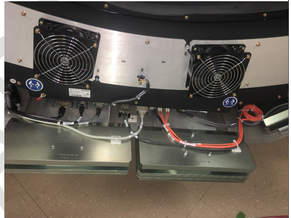
Figure 44 – DMS Fans (number of fans and locations may vary from that shown)
