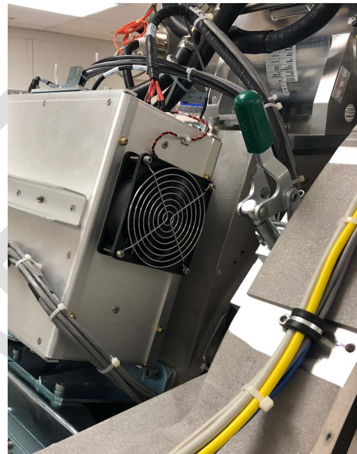
Figure 46 – Fan on rear of Aux box
